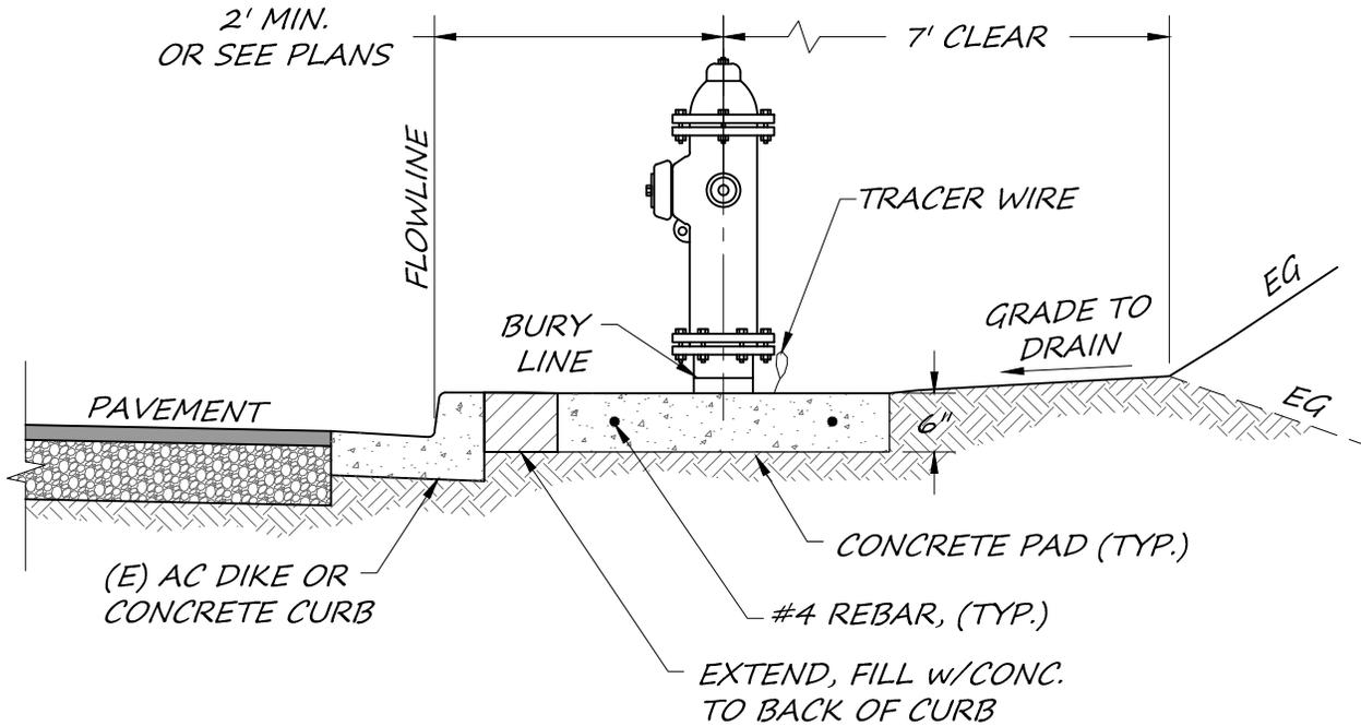
**AT VERTICAL CURB AND GUTTER, (NO SIDEWALK)**
