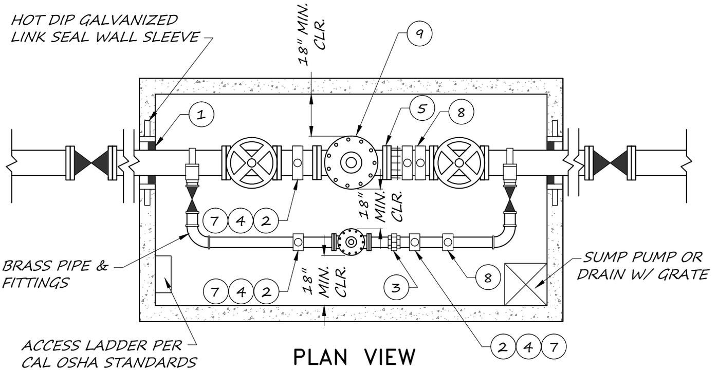
VAULT SHALL HAVE FULL OPERATING SPRING ASSISTED TRAFFIC RATED LID WITH STAINLESS STEEL HARDWARE & PADLOCK LOCKING LATCH.
