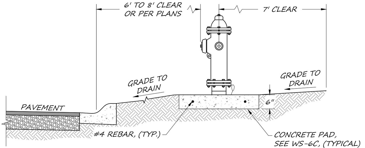
**AT ROLLED CURB AND GUTTER (NO SIDEWALK)**
